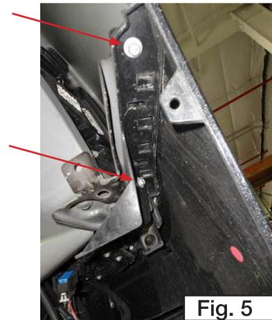
8. Carefully depress the two clips holding the plastic bumper support to the fender (Fig. 6). Pull down on the plastic support in order to remove it.
