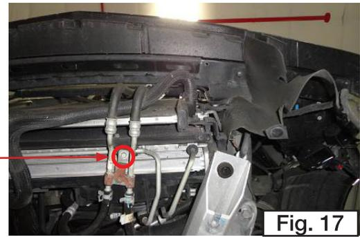
20. Using the provided red plastic plugs, remove the oil cooler lines from the oil cooler and plug the lines and oil cooler to prevent oil from leaking (Fig. 18).
